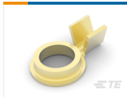
TE Part #160088-3 RING TONGUE 20-16 AWG 0.198 X . 700 BR
