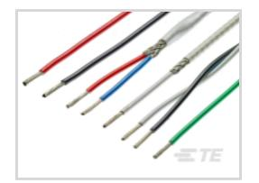
Cable Type: Spec 99M Voltage Rating: 600 V Wire & Cable Insulation Material: Radiation-Crosslinked, Modified Polyester Conductor Material: Tin-Plated Copper Wire Size: 22 AWG
