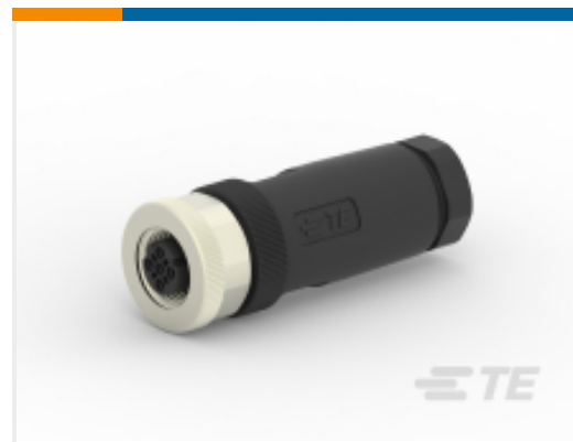
TE Part #T4110502041-000 M12,FEMALE,STRAIGHT,D CODE,4P, PG9,GOLD
