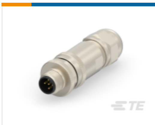
TE Part #T4111012051-000 M12 M, 5P GOLD A_CODE S SHIELDED PG9
