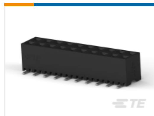
TE Part #2-2307819-0 20P,2MM,BB,REC,DRVT,SMD,AU.76, TR,W/CP
