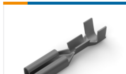
TE Part #150346-2 110 MINI FASTON,REC.,24-20 AWG, TPBR
