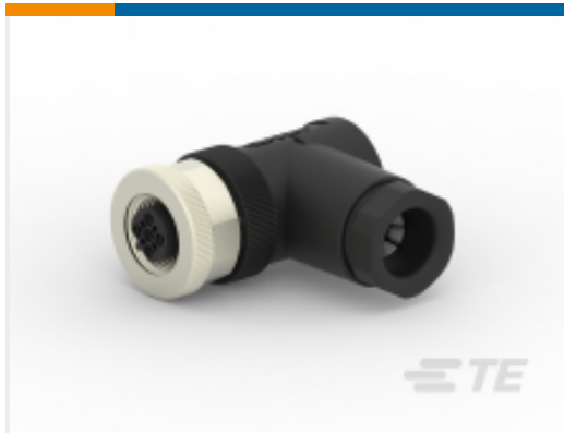
TE Part #T4112402051-000 M12,FEMALE,RA,B CODE,5P,PG9, GOLD
