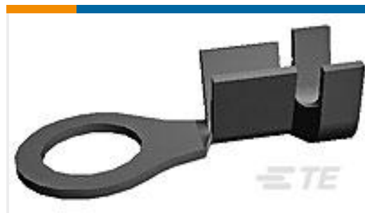
TE Part #40955 RING 20-16 AWG .0295 X .390 TPBR
