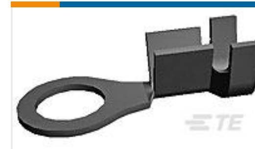
TE Part #160101-9 RING TONGUE 20-16 AWG 0.0253 NPBR
