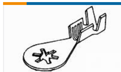
TE Part #3-521013-2 ULTRA-FAST 250 ASY REC 16-14 AWG TPBR
