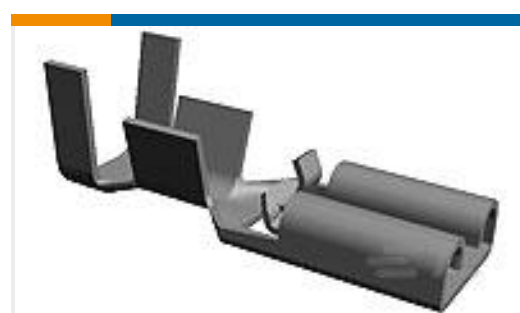
TE Part #1217113-1 PL 187 TERMINAL RECEPTACLE 22-18 AWG BR
