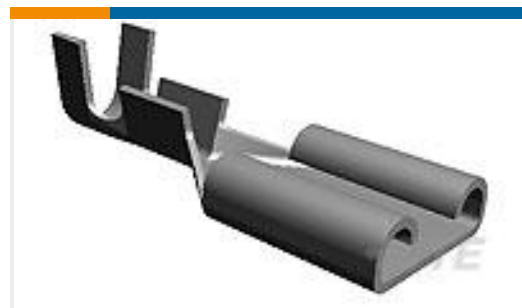
TE Part #42617-1 187 FASTON REC 20-16 AWG BR
