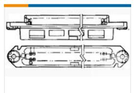
TE Part #2-552001-1 ASSY, RCPT, 50 POS, B SLOT
