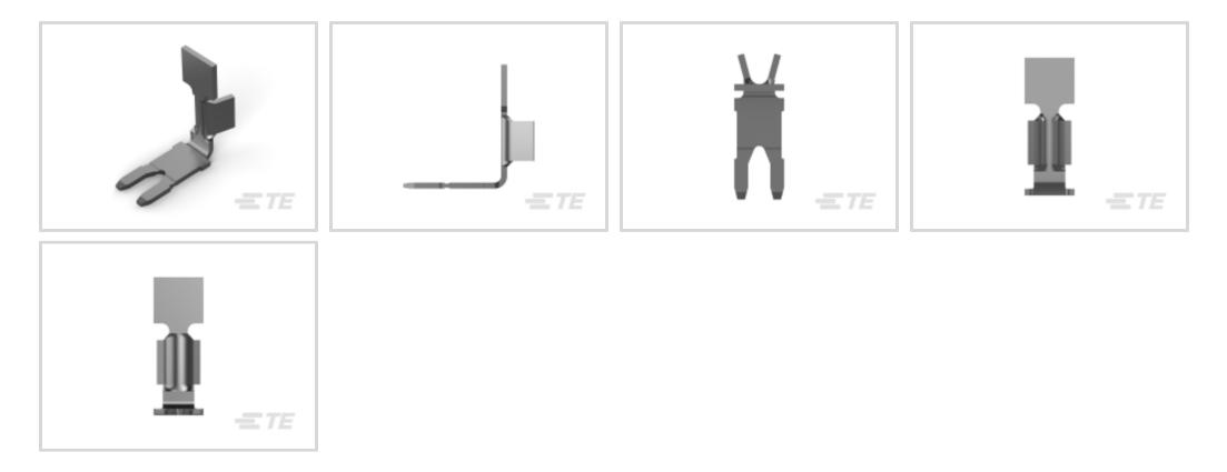
Magnet Wire Terminal Type: Poke-In Mating Tab Width: 3.04 mm [.119 in ] Mating Tab Thickness: .46 mm [.018 in ] Lead Wire Size: .3 – .8 mm<sup>2</sup>
