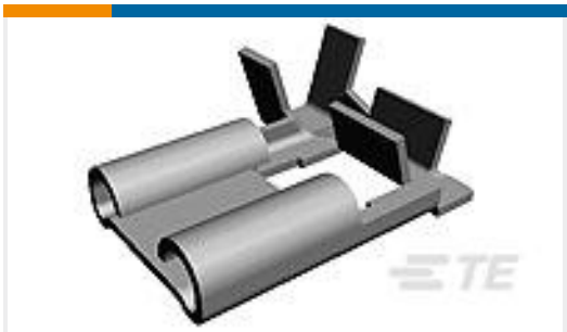
TE Part #63010-2 250 FASTON FLAG REC 18-14 AWG TPBR
