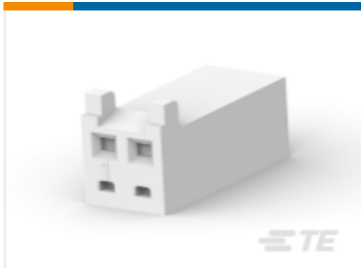
TE Part #1375820-2 Receptacle Housing: 2.54mm, 1 Row, CST-100 II
