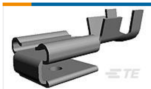
TE Part #62253-2 250 FASTON REC 14-10 TPBR
