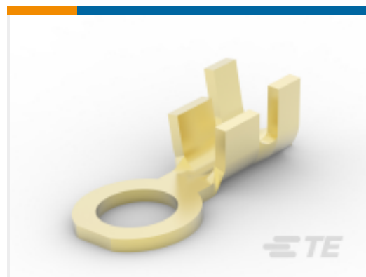
TE Part # 61764-1 RING CRIMP 20-16 AWG BR
