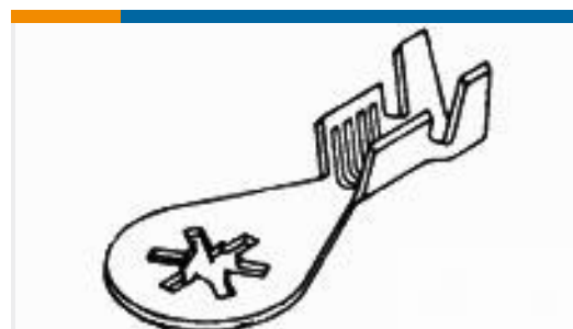
TE Part #62612-2 RING .164 12-10 AWG 0245 TPCRS
