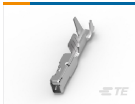
TE Part #2098762-4 Contact,female0.64, 22 AWG, CuNiSi, Sn
