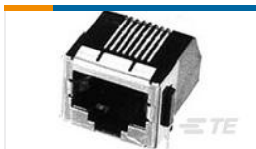
TE Part #5555141-1 MJ,LPF,R/A,8P/8C,SHLD,PNL GRD
