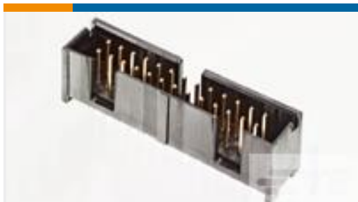
TE Part #5650479-5 ASSY,PIN,EUROCARD,TYPE R/2,LEAD-FREE,48
