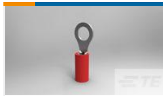
TE Part #171508-2 PIDG WIRE TERM, #8, 22-16 AWG
