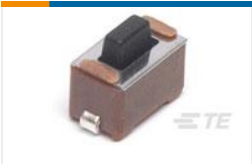
TE Part #147873-1 SWITCH,TACT,SMT,J-LEAD,5.0MM
