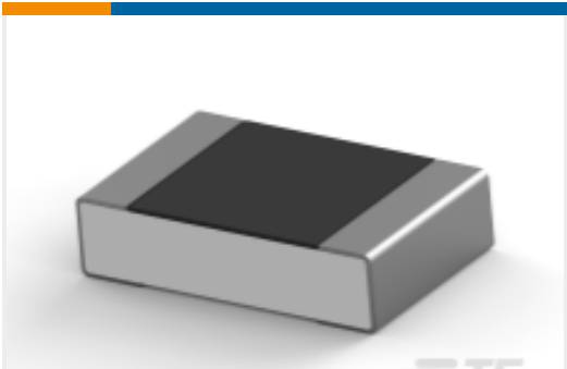
TE Part #5-2176380-3 RQ 0805 4K02 0.1% 10PPM 5K RL
