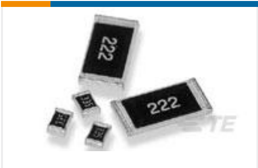
TE Part #1623149-1 CRG0805 1% 20K
