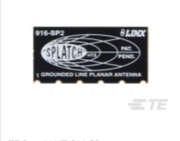
TE Part #ANT-916-SP Antenna SP PCB RPC 916MHz SMT
