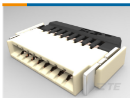
TE Part #1-2328702-0 10PIN 0.5MMP FPC CONN, BACK FLIP LOCK
