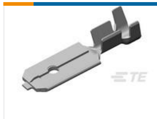
TE Part #626378-1 250 FASTON TAB 18-14 AWG BR
