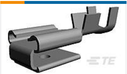
TE Part #61944-2 250 FASTON REC 18-14 AWG TPBR
