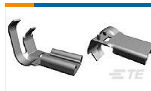
TE Part #1742543-1 250 FASTON, FLAG, REC., 18-12 AWG, NPST
