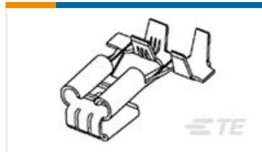
TE Part #151321-4 250 FASTON,FLAG,REC.,18-14 AWG, TPBR
