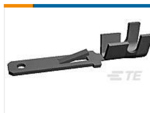
TE Part #60294-2 FF 250 TAB 22-18 AWG .032 TPBR
