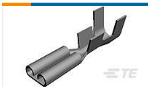
TE Part #60635-3 250 FASTON REC 14-10 AWG BR
