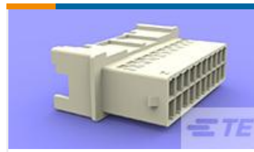
TE Part #1969592-8 HSG,REC,FREE-HANGING,DUALROW, EP2.5
