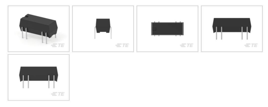
Contact Voltage Rating: 24 VDC Signal Relay Coil Power Rating (DC): 34 mW Isolation (HF Parameter): -18dB @ 900MHz, -30dB @ 100MHz Insertion Loss (HF Parameter): -.12dB @ 100MHz, -1.9dB @ 900MHz Signal Relay Mounting Type: Printed Circuit Board
