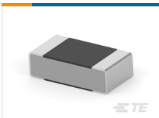
TE Part #6-1879207-9 RN 0603 511K 0.1% 10PPM 5K RL
