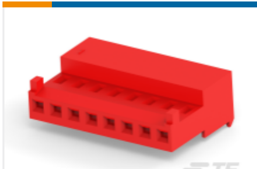
TE Part #3-644042-8 Nylon Gold Plated Receptacle: 2.54 mm, with Mating Alignment, MTA 100
