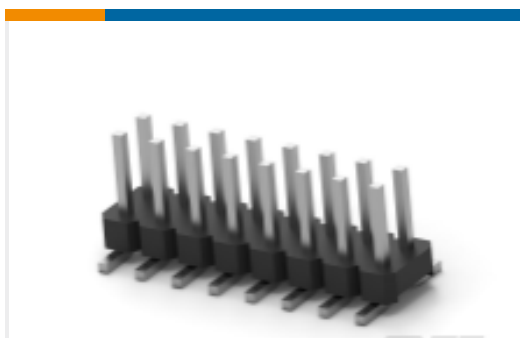
TE Part #2842142-7 14P,2MM,BRK HDR,DRVT,SMD,0.1AU, TR W/CAP
