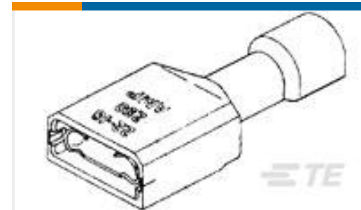
TE Part #9-520193-2 ULTRA-FAST 187 ASY REC 22-18 AWG TPBR
