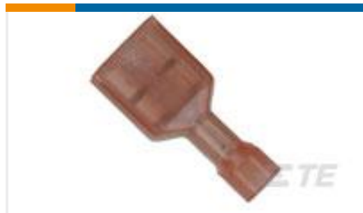
TE Part #4-521097-2 ULTRA-FAST 250 ASY TAB 12-10 AWG TPBR
