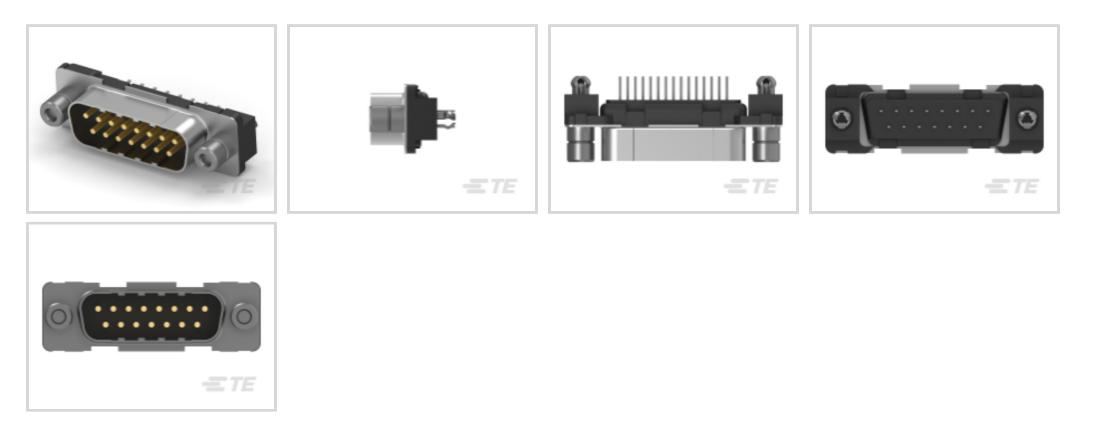
Connector & Housing Type: Plug Connector System: Cable-to-Board Number of Positions: 15 Centerline (Pitch): 2.74 mm [.108 in] Number of Rows: 2
