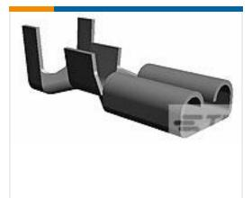
TE Part #170038-2 187 FASTON,REC.,20-16 AWG,TPBR
