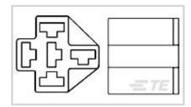
Relay Socket Type: Wiring Harness Relay Socket For Use With: Plug-In Mini ISO Relays
