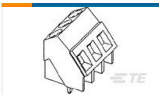
TE Part #1-1546074-2 12POS 5.08MM TERMI-BLOK TOP WI
