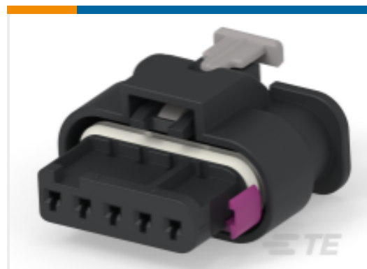
TE Part #1-2355515-5 5POS, MCON 1.2, REC HSG ASSY, SLD, COD A
