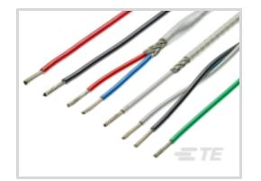
Cable Type: MIL-DTL-81044 Voltage Rating: 600 V Wire & Cable Insulation Material: Modified Radiation Cross-linked PVDF Conductor Material: Tin-Coated Copper Wire Size: 26 AWG
