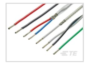
Cable Type: MIL-DTL-81044 Voltage Rating: 600 V Wire & Cable Insulation Material: Modified Radiation Cross-linked PVDF Conductor Material: Tin-Coated Copper Wire Size: 16 AWG
