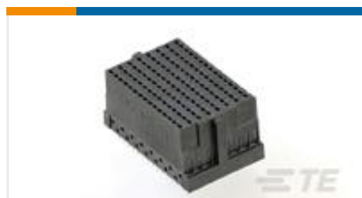
TE Part #1-1871058-5 PCI EXPRESS CONN. EON TYPE, 280P, L=3.25
