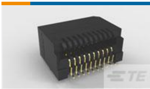
TE Part #1888247-1 20 POS SMT CONN, SFP/SFP+, 30A
